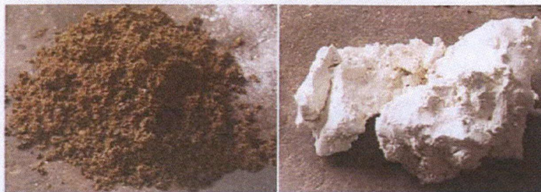
Components of premixed 'wet' mortars – well graded, sharp sand and fat lime putty
