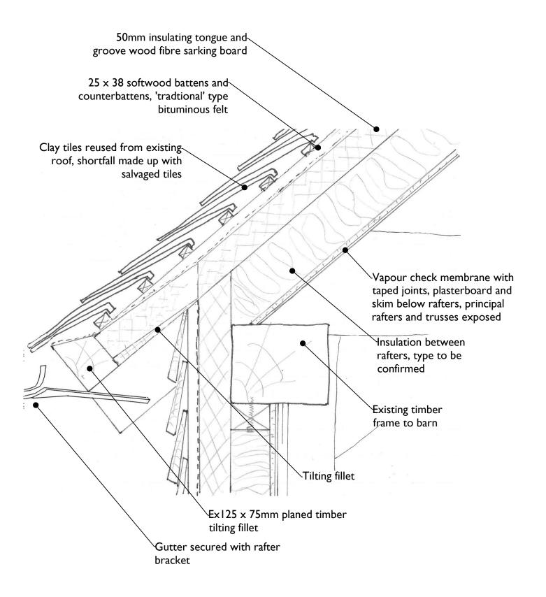
SECTION THROUGH EAVES TIMBER CLAD SECTION
