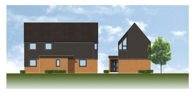
Illustration of a typical 2 storey HMO dwelling with a simple palette of materials: red brick cladding to ground floor, and black stained timber cladding to upper floors topped with dark grey / black roof slates.
