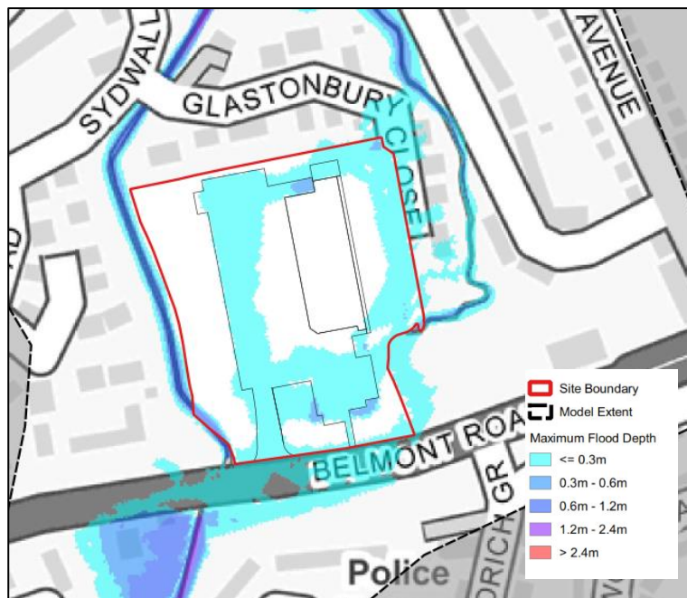
Figure 5 – 67% Belmont Road Culvert Blockage - 1% AEP plus 37% CC – Flood Depths (Proposed)
