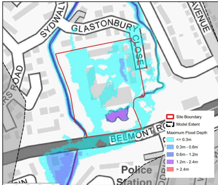
Figure 4 – 67% Belmont Road Culvert Blockage - 1% AEP plus 37% CC – Flood Depths (Existing)
