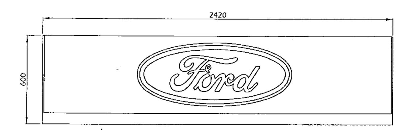
O/A SIZE OF SIGN 2420mm x 600mm O/A WEIGHT OF SIGN 31.5Kg
