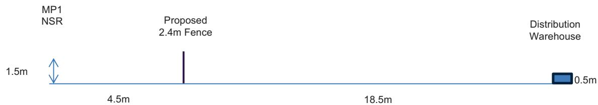
The activity sounds were generally at ground level. Vehicle sound source height is taken as 0.5m from the road surface (CRTN, 1988). The greater and more onerous height of 0.5m is used.
