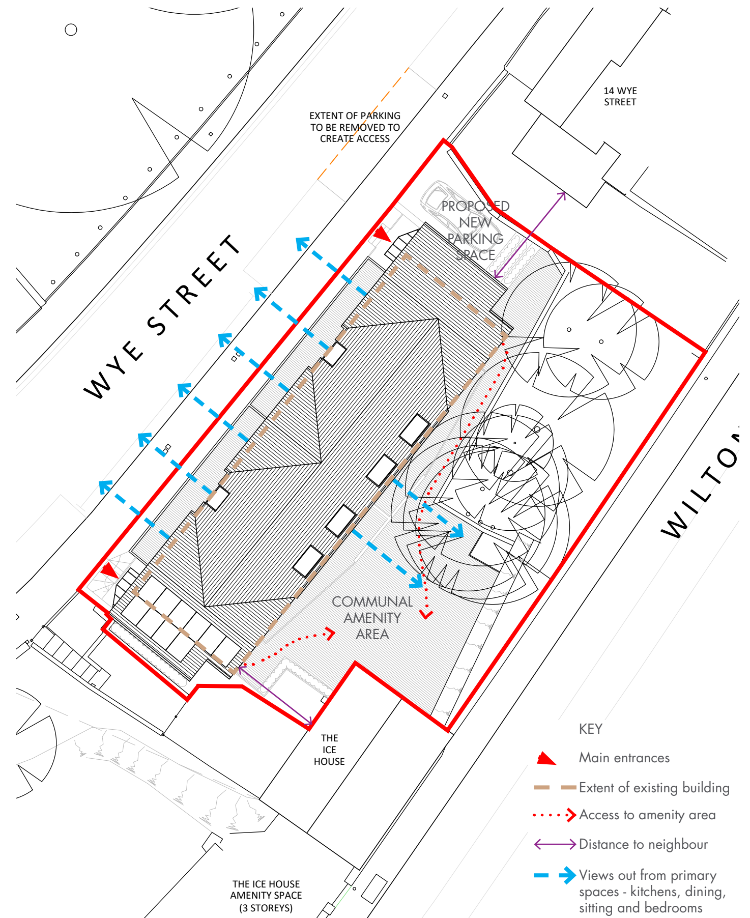
Image 30 (right): Proposed Site Plan showing access into and through the building, and views out from primary spaces
