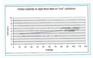
A series of collision types at high risk locations where Y distance was less than 45m were compared with locations with more than 45m visibility. There were no statistically significant differences between the two sets of data. The data analysed included main road bus and large goods vehicle collisions, and the research did not find high numbers of collisions involving these types of vehicles at low visibility sites.
