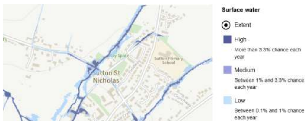
Figure 2: EA Surface Water Flood Risk Mapping.
