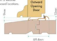
NOTE: Door/Entrance Frames are delivered to site with threshold supplied loose, for on-site fixing. Actual threshold may differ from one shown. Door Frame sizes shown are nominal and are approx 5mm less than the size shown to allow for building in.
