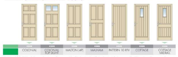
NOTE: All fully finished door and entrance frames must be fitted using cleat fixing (see installation manual). All the above frames can be supplied in imperial sizes - prices on application. Door Frame sizes shown are nominal and are approx 5mm less than the size shown to allow for building in. All illustrations above tables show exterior views.
