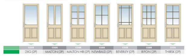
NOTE: All fully finished door and entrance frames must be fitted using cleat fixing (see installation manual). All the above frames can be supplied in imperial sizes - prices on application. Door Frame sizes shown are nominal and are approx 5mm less than the size shown to allow for building in. All illustrations above tables show exterior views.
