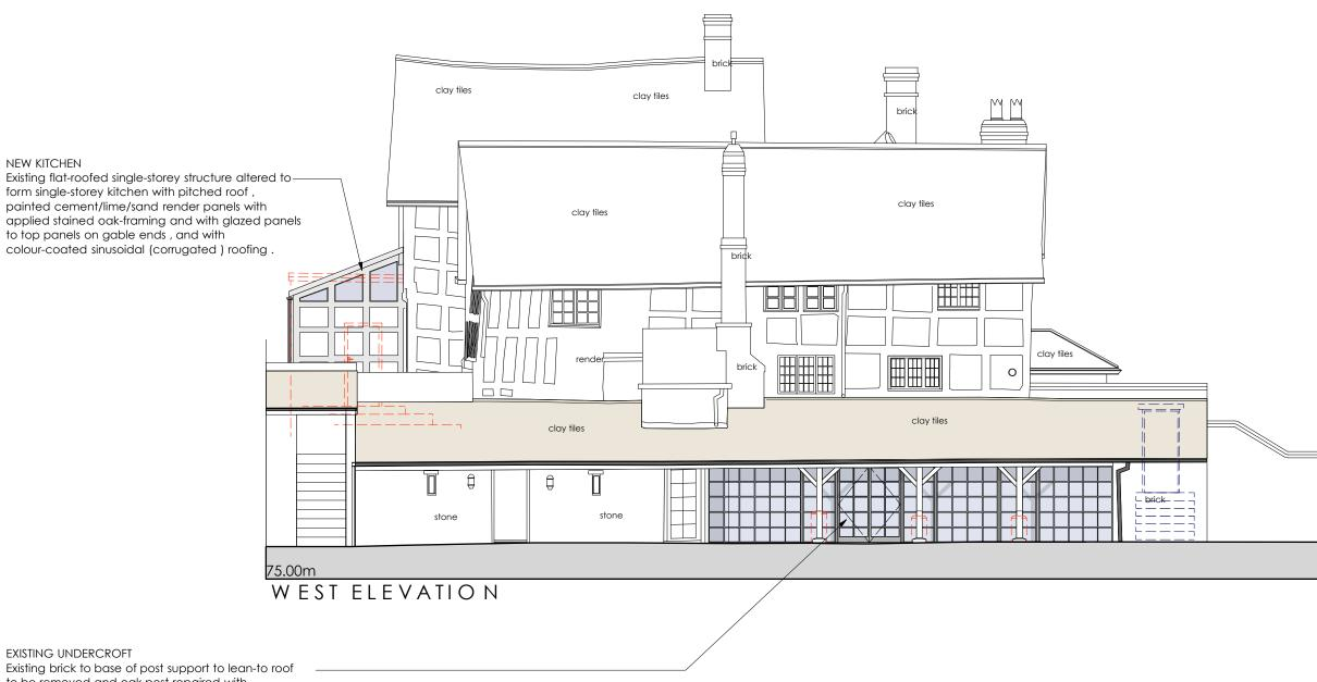
to be removed and oak post repaired with matching section extended to new staddle stone base with 20mm dia stainless steel location pin between stone and oak. New glazed infil panels behind posts in stained
