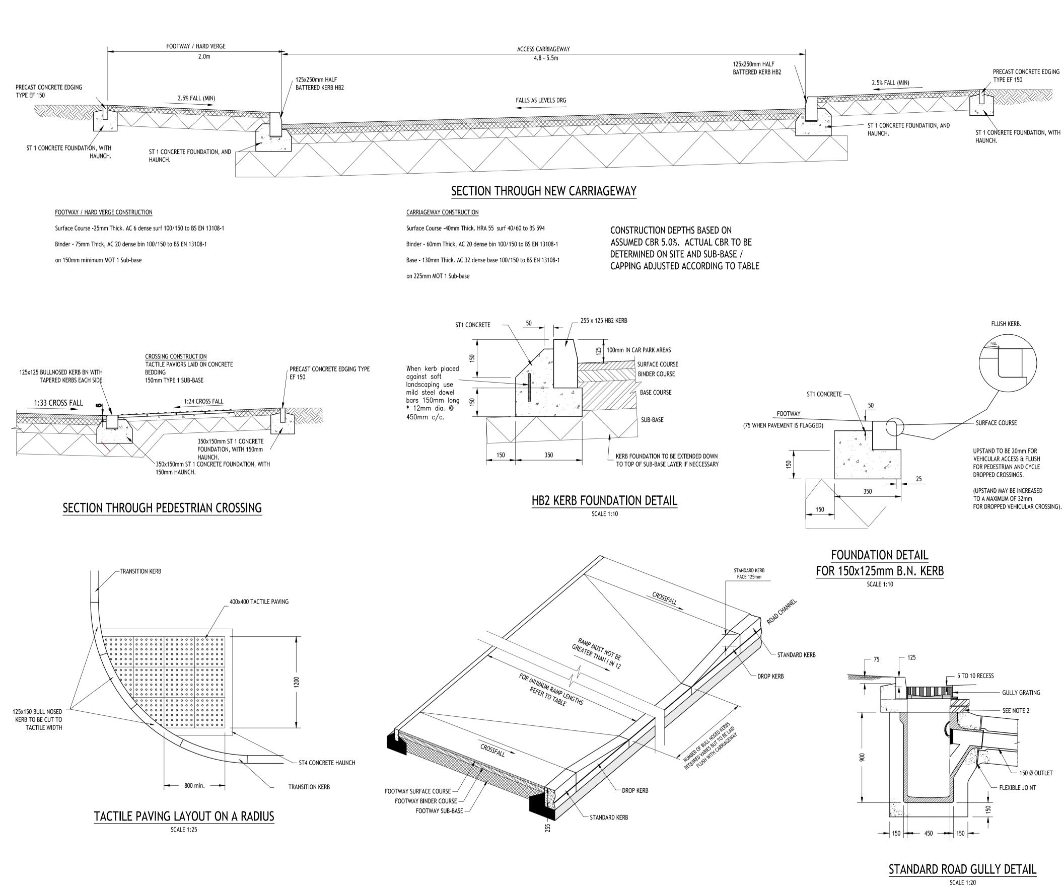
CARRIAGEWAY FOOTWAY - 125x125 BULLNOSED KERB BN 350x150mm ST 1 CONCRETE FOUNDATION, WITH 150mm HAUNCH.
