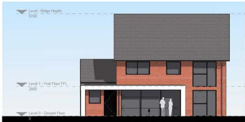
Elevation C - Rear Elevation 1 : 100
