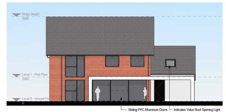
Elevation C - Rear Elevation 1 : 100
