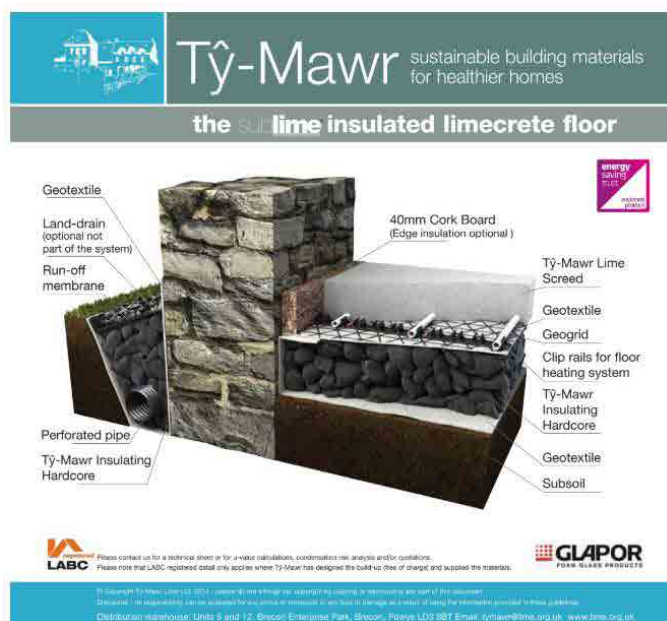
Figure 1: Ground Floor Build-up - As be Ty Mawr system. SumLine insulated limecrete floor. Including UFH. GF approx 9sq m
