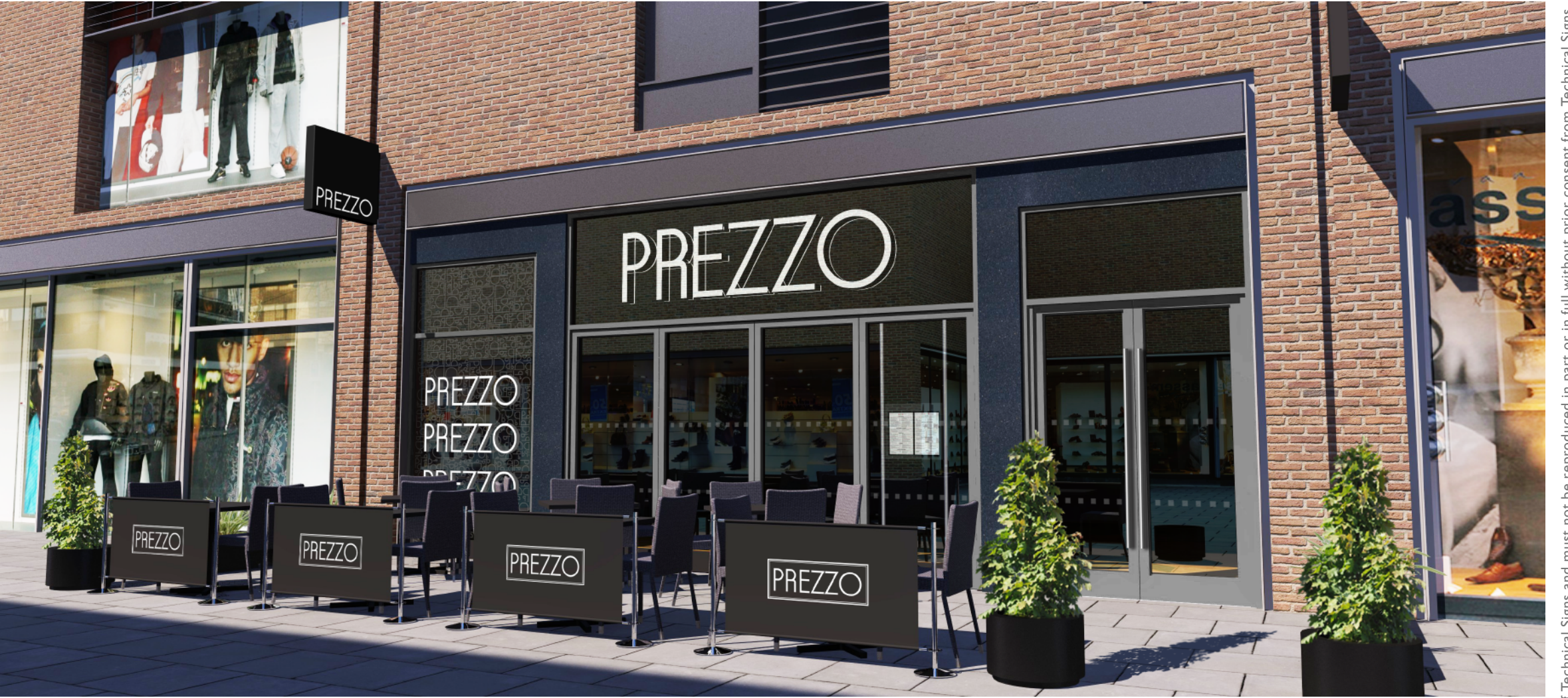
Proposed: Built up face illuminated letters bonded to the inside of the glass above the shopfront. Internally illuminated pole mounted menu box. Digitally printed 'P' window vinyl with three sets of face illuminated text bonded to the inside of the glass. Internally illuminated porjection sign.
