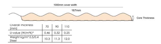
The KS1000 SRW insulated roof panels have a Thermal Transmittance (U value), calculated using the method required by the Building Regulations Part L2 (England & Wales) and Building Standards Section 6 (Scotland).
