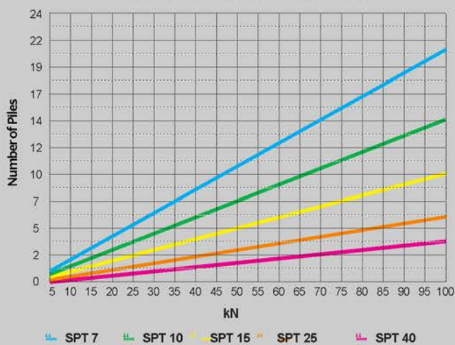
COMPRESSION - PILES L=2m [60,3 mm]
