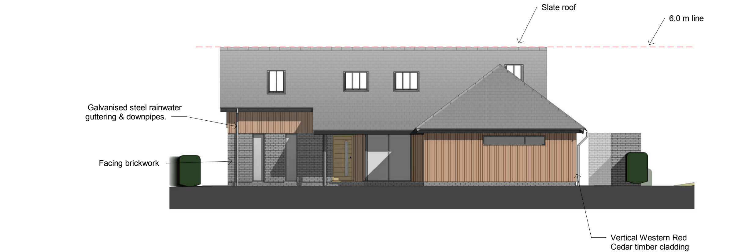
North West Elevation. 1 : 100
