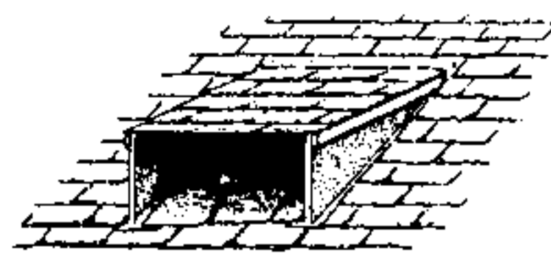
Ridge ventilators can be adapted as bat access points. It may be necessary to remove internal mesh or plastic mouldings.
