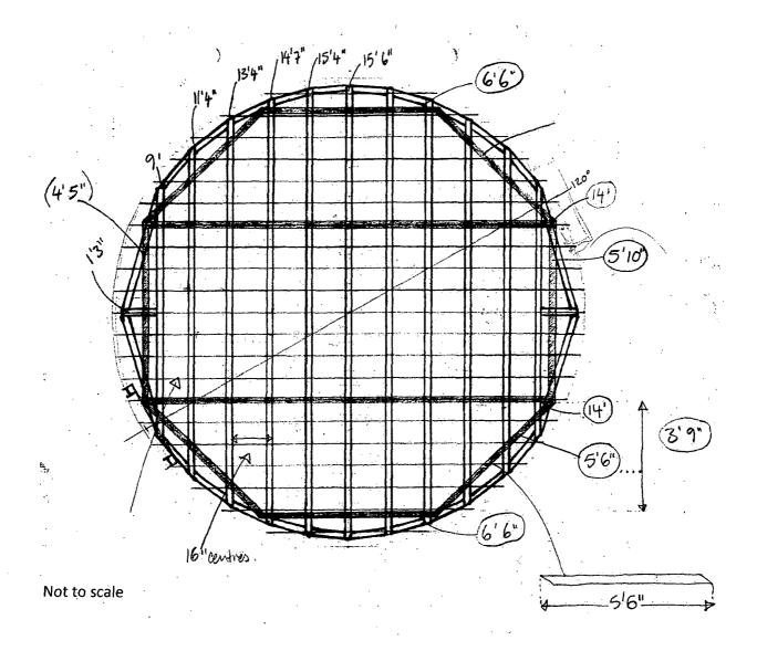
Sample plan of decking for a yurt with diameter of 16 feet.
