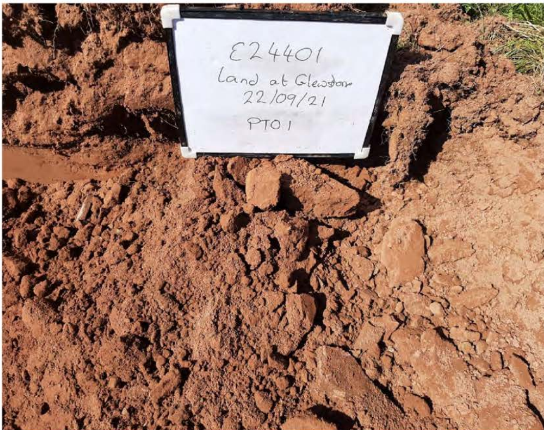
Photo 10: Percolation Pit PT01 Spoil
