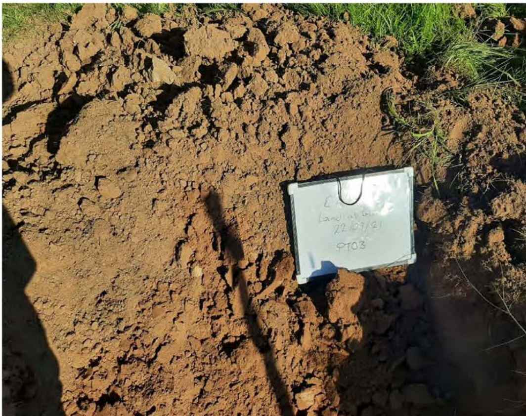
Photo 14: Percolation Pit PT03 Spoil
