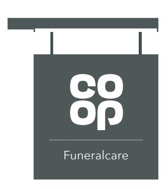
1No. Externally illuminated Projection sign, powder coated RAL Grey 7010, lettering to be White. Illuminated via troughlight.
