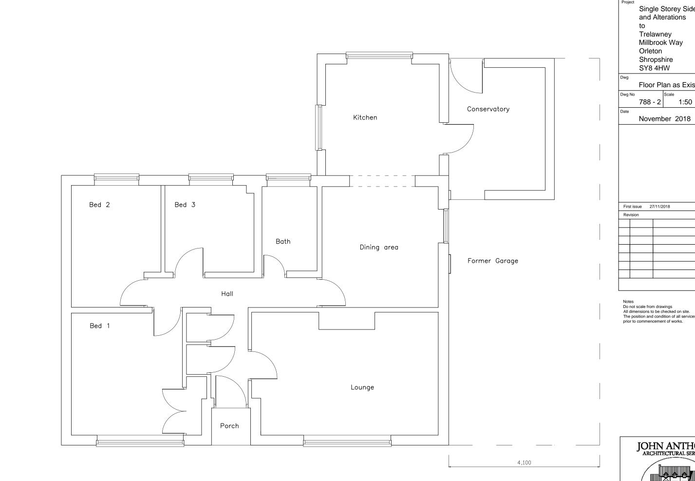
Single Storey Side Extension and Alterations Floor Plan as Existing Paper Scale A3
