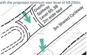
As discussed, minimum weir level will be updated to **65.35**. This will represent the as built levels and will remain lower than the cycleway as requested (as built cycleway level 65.41). Please see attached as built survey for your information.
