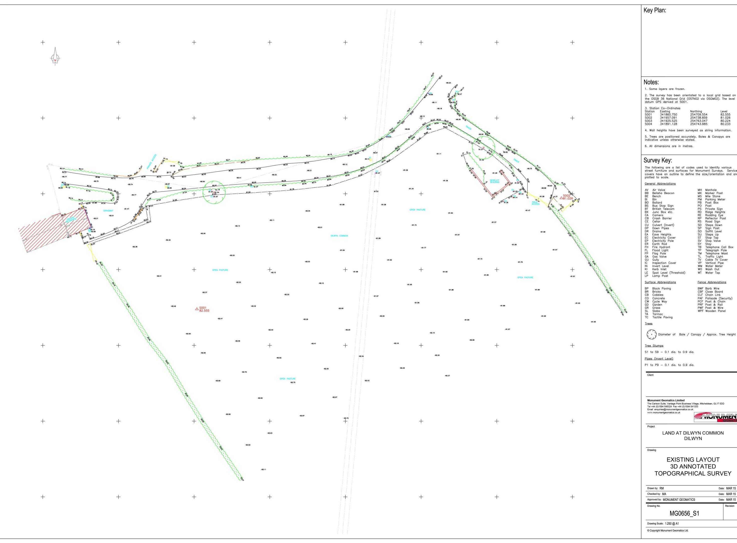
2. The survey has been orientated to a local grid based on the OSGB 36 National Grid (OSTN02 via OSGM02). The level datum GPS derived at S001.
