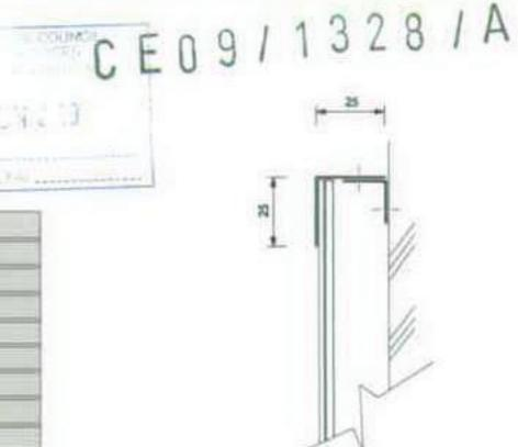
EXTERNAL SERVICES PANEL CONSTRUCTED FROM 5MM RIGID SHEET FACED WITH EXTERIOR QUALITY DIGITAL PRINT AS SHOWN.
