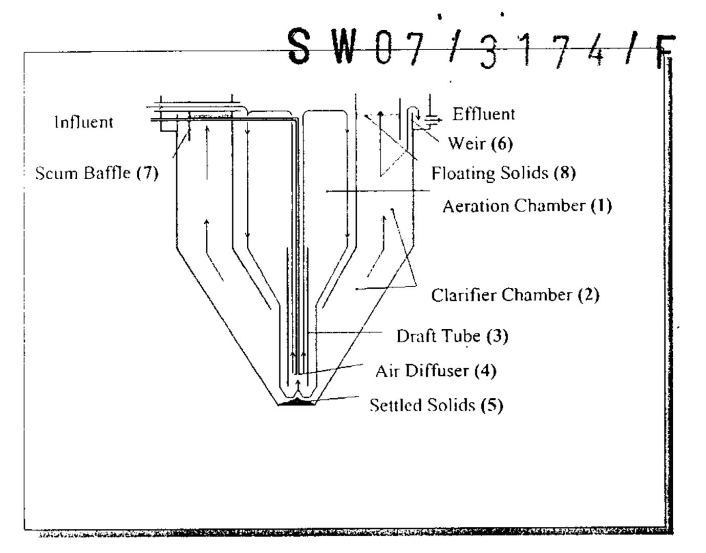
The Diamond system consists of two treatment chambers within a single tank.
