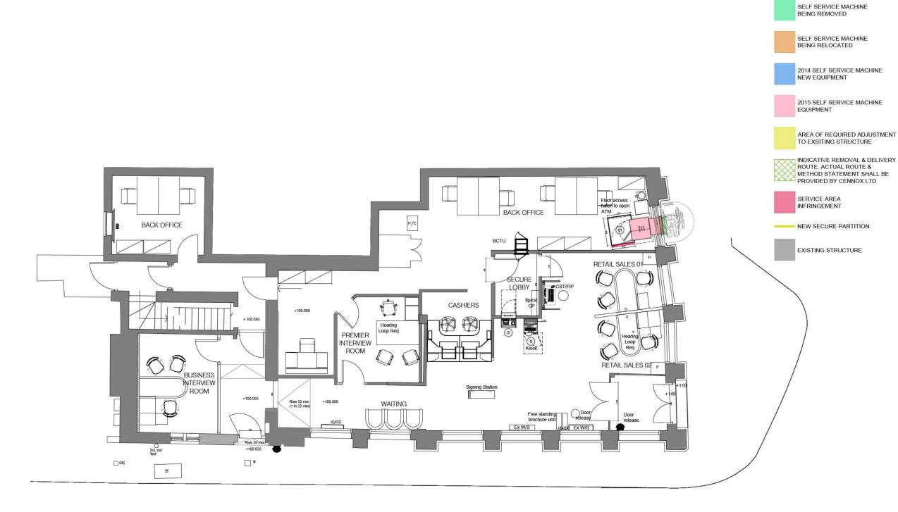
PROPOSED BRANCH LAYOUT INCLUDING REMOVAL & DELIVERY ROUTE (scale 1:100 @ A3)
