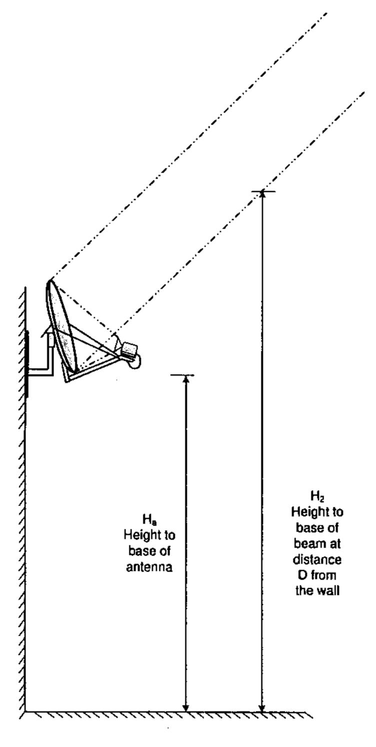
When installed, the antenna seems to be pointing lower in the sky than the direction the radio energy is actually transmitted. This energy tends to stay within a tube the size of the antenna until it reaches something called the collimation point where it will then spread out a little. The collimation point for our antennas will be in excess of 50m from the VSAT antenna.
