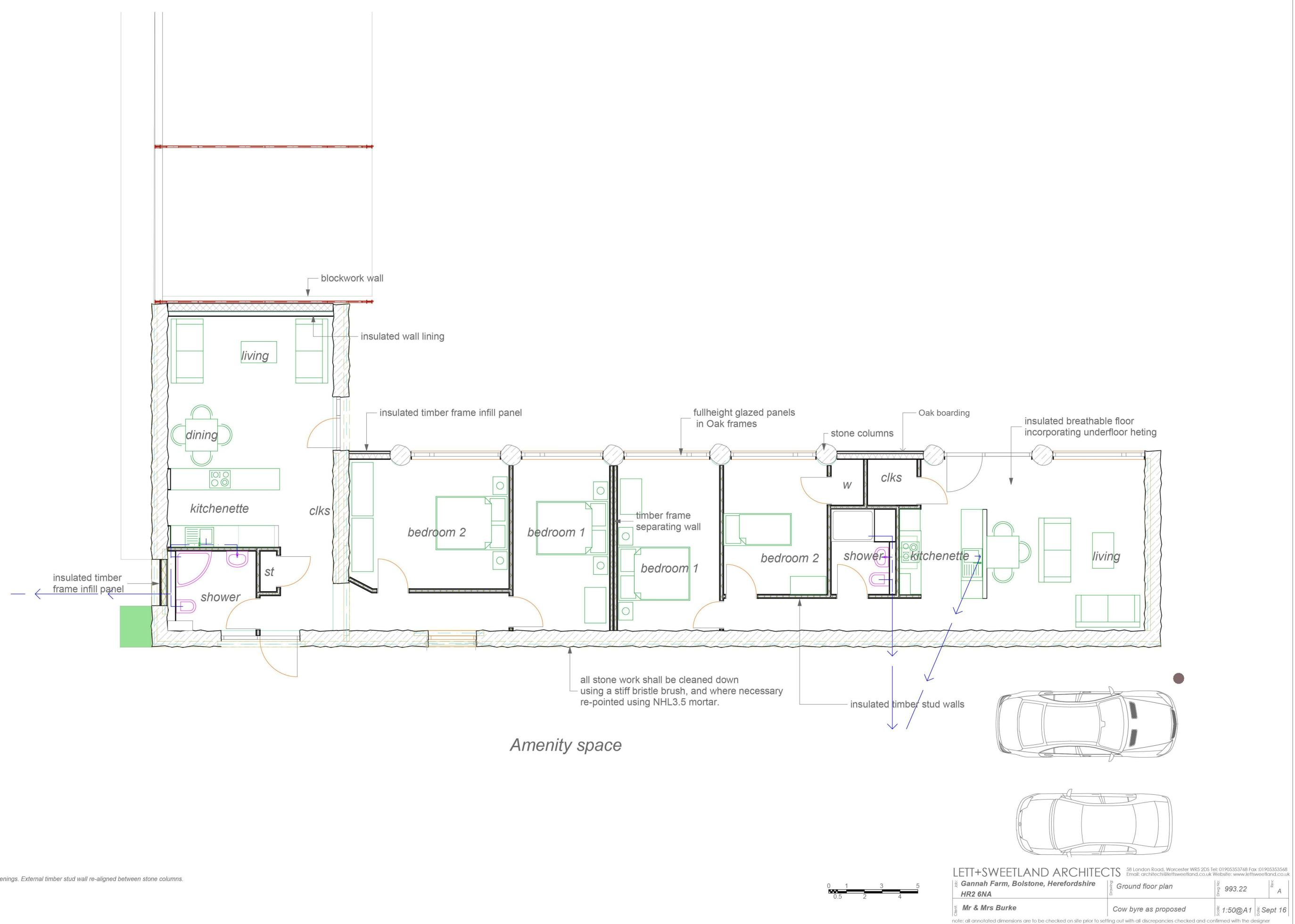
Rev A: Window and doors set further backl into openings. External timber stud wall re-aligned between stone columns. Joinery noted as Oak. 28.7.17
