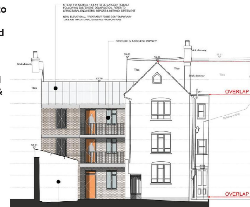
Right: Rear elevation showing the proposed reconstructed no. 18 & 19
