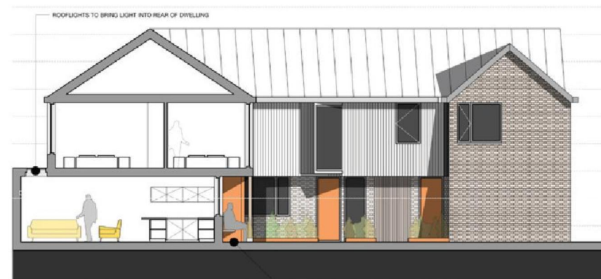
02 PROPOSED NEW BUILD DWELLINGS WEST ELEVATION - SHOWING SECTION THROUGH UNIT NB04 1:100
