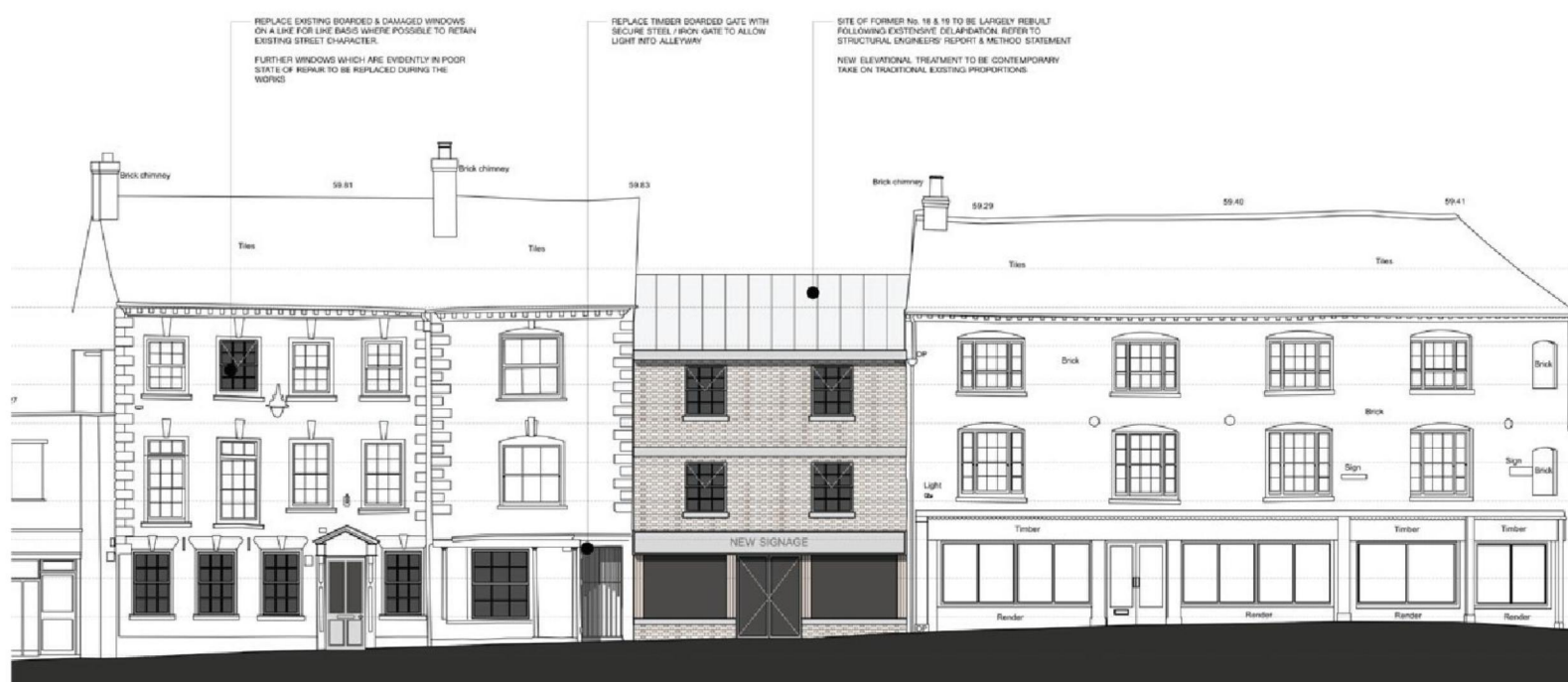
Left: Street Elevation to High Street showing reconstructed facade to no. 18 & 19
