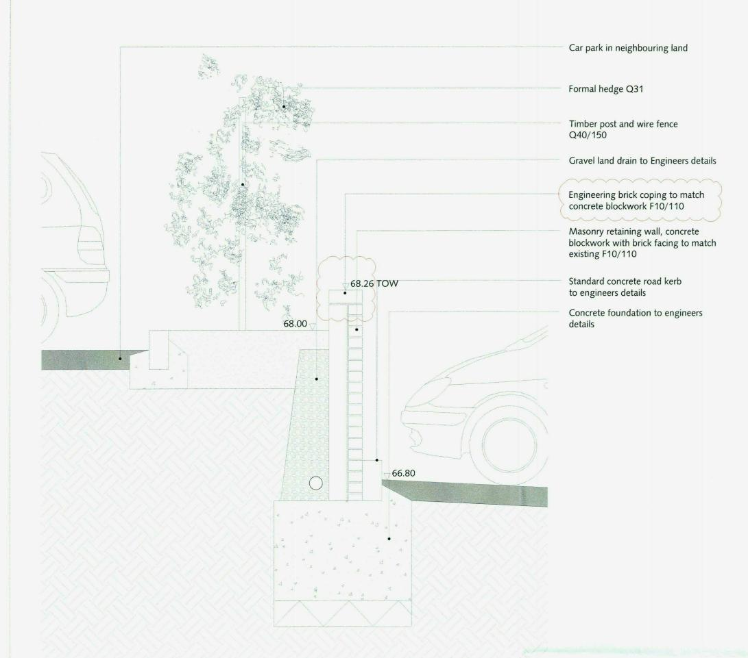
2 Typical Section A-A Scale 1:20
