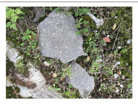
Photo 11: Bituminous ACM fragments used as roadway surface dressing.
