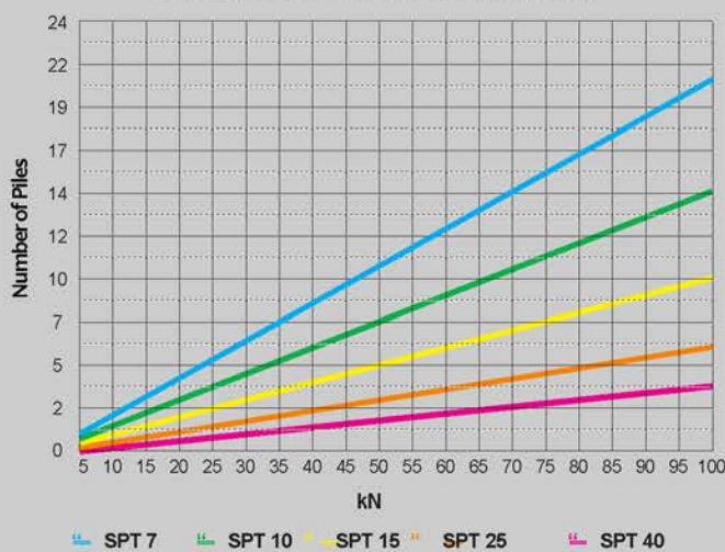
COMPRESSION - PILES L=2m [60,3 mm]
