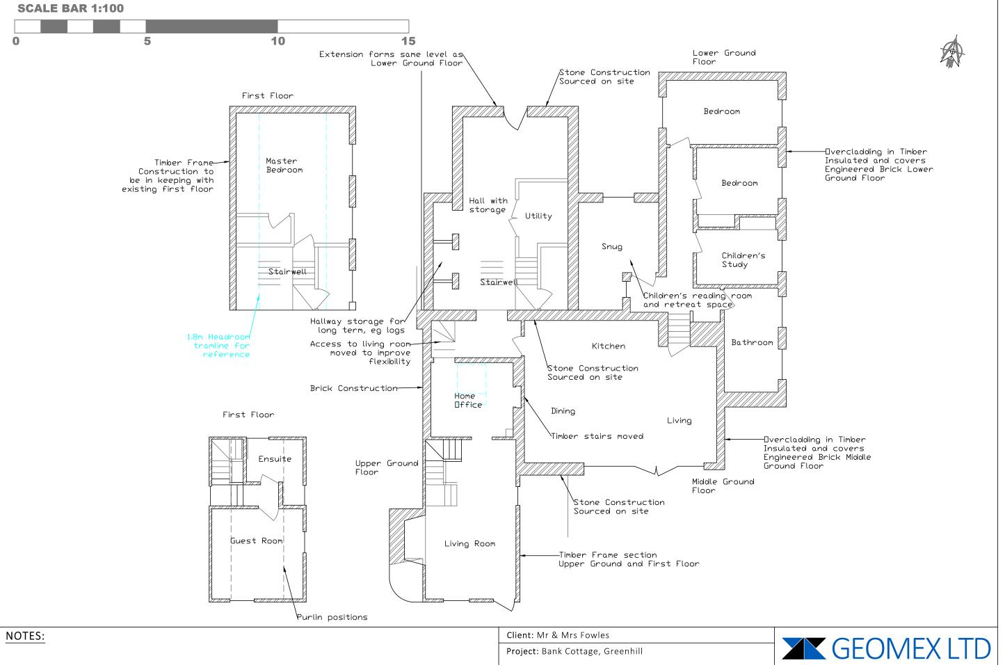
**Drawing Title:** Proposed Floor Plan Drawing No: BCG-PFP-JEBB Revision: 000 Date: May 2023 Drawing Scale: 1:100 @ A3 NOTE: ALL DIMENSIONS TO BE CHECKED ON-SITE
