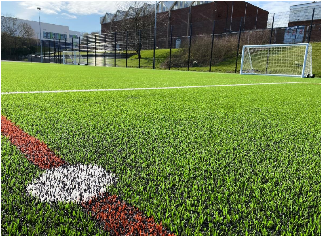
3G synthetic turf surface, designed to look, play and feel as close to natural turf as possible.
