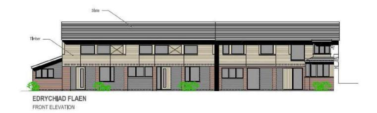
In reference to the existing workshop building, there will be no changes to heights as it is the intention of the proposal to work within the confines of the existing fabric. Material alteration of doors and windows will be made, but as a whole, the scale and façade context will remain as. The proposal also creates a single storey extension to the south end wall to the workshop and is suggested to treat this as a "lean to" which is typical of vernacular architecture.
