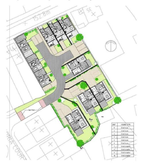
Speed into Deacons Yard will be controlled at the junction with Victoria Court, by the inclusion of one ramp, thus reducing speed to a maximum of 15 mph. Whilst the general topography of the site is level, by pure identification that the surfaces are
